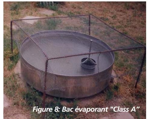
Figure 8: Bac évaporant "Class A"
